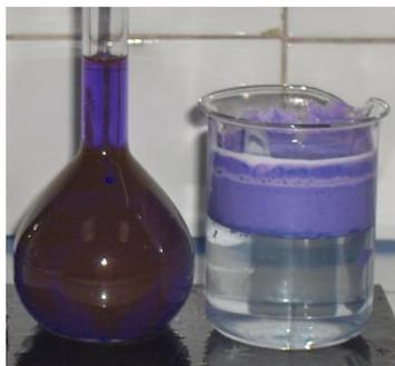
Fig. 7 - Dye mixture solution containing MB, RhB, MG and BR29 before and after extraction by ELM under most favorable experimental conditions (the concentration of each dye in the mixture is 10 mg/L).
