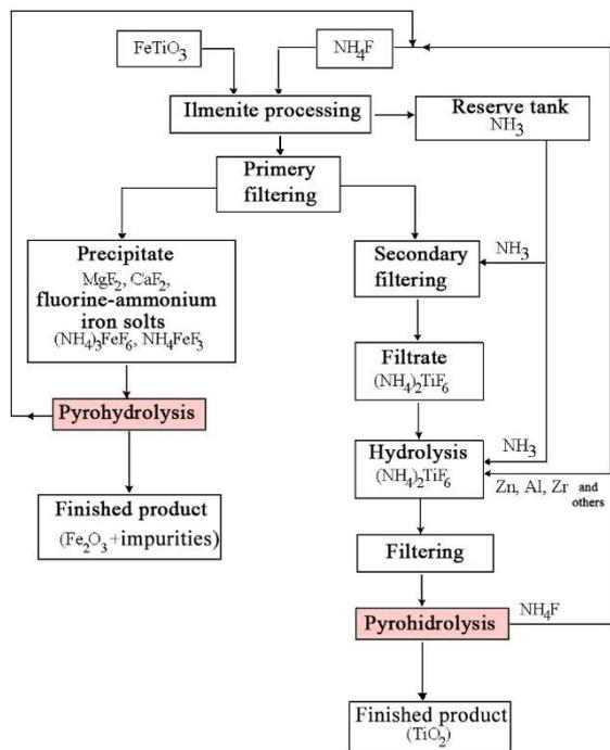
Fig. 2 - Scheme of technological operations in the hydrofluoride process for the production of titanium dioxide and iron oxides.
